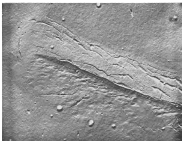
Fig. 25. Surface of Van Arkel zirconium after 10 hr in steam at 1 atm, 500°C, showing pustule (Formvar/carbon replica, shadowed Pd/Au). Magnification approximately 4000X.
