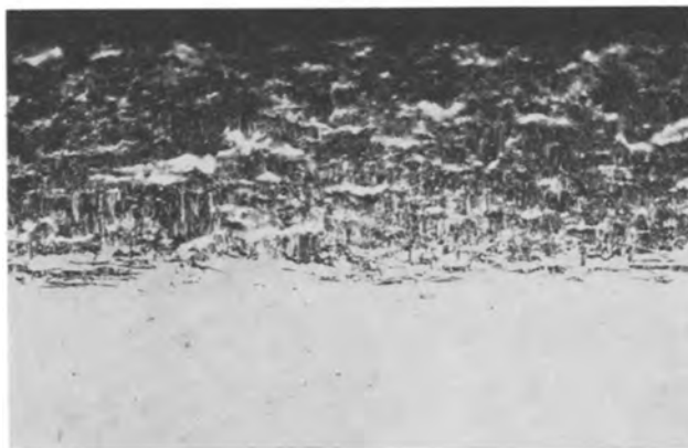
Fig. 12. Metallographic cross section of tantalum specimen oxidized for 2300 min at 900°C and 0.01 Torr O 2 . Magnification approximately 120X. (a) (top) Vertical illumination; (b) (bottom) polarized light.
