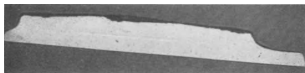
Fig. 5. Polished and stained cross section of an InSb dendrite showing a degenerate twin plane lamella. Magnification approximately 50X.
