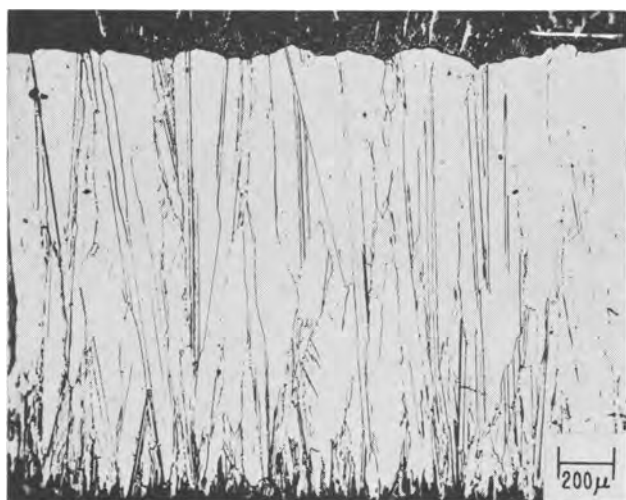
Fig. 1. Cross section of copper electrodeposit, 1700 \mu thick, showing growth twins. Substrate at bottom. Etching reagent: ammonium hydroxide and hydrogen peroxide.
