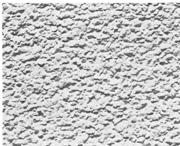
Fig. 7. Surface of CdTe film 5000Å thick, deposited at 200°C. Magnification 10,000X before reduction for publication.
