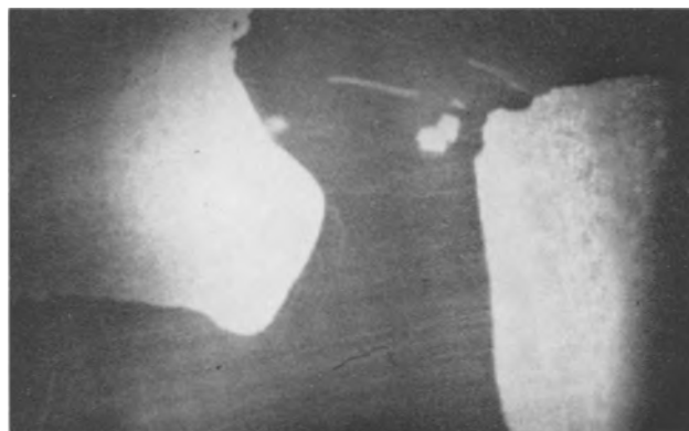
Fig. 10. Appearance of 55 amp arc photographed at high speed. Time interval represented is 0.0007 sec. Anode is at the right of the photograph. Magnification approximately 7X.
