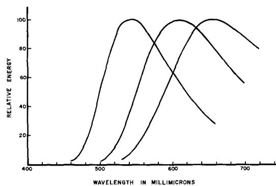
Fig. 4. Emission spectra of SiC crystals at room temperature under 3650Å excitation. (The ordinate is relative energy per unit wavelength interval.)
