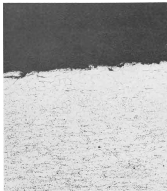
Fig. 5. Transgranular attack in Zr inhibited loop. Magnification 250X.
