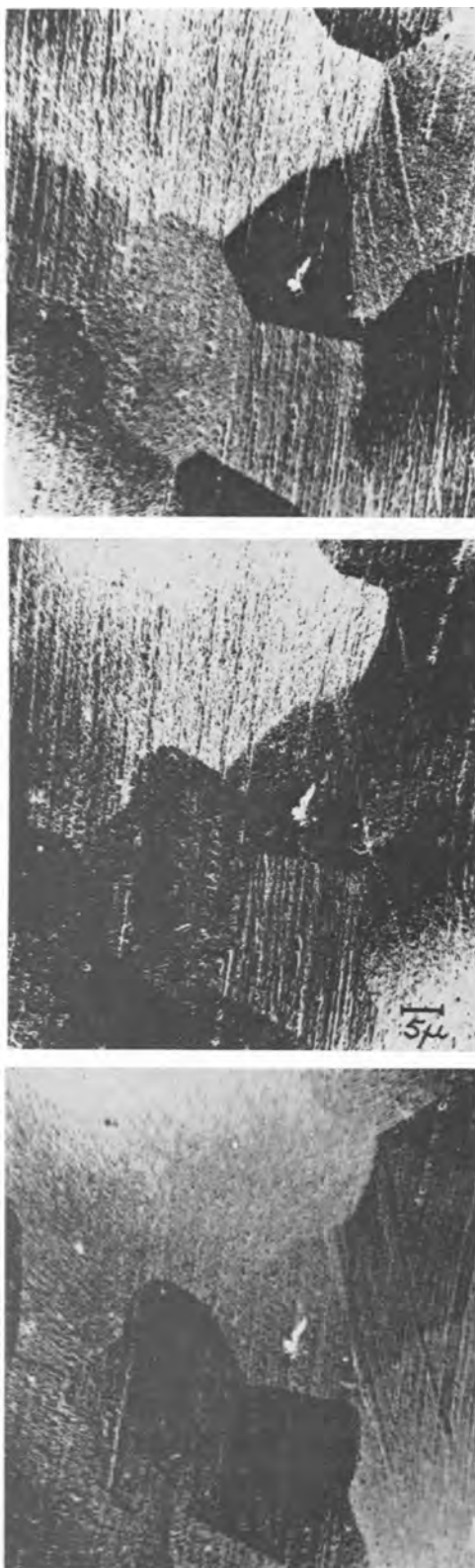
Fig. 2. Effect of tilting specimen relative to incident electron beam: 2a (top) +10^\circ tilt; 2b (center) 0^\circ tilt; 2c (bottom) -10^\circ tilt. Magnification approximately 1000X.
