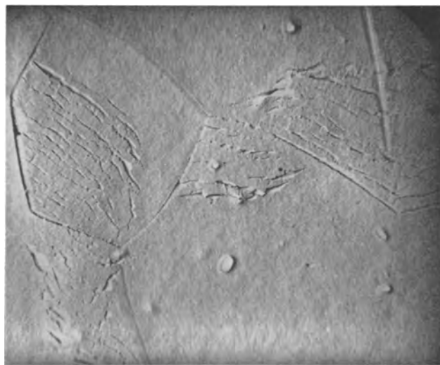
Fig. 23. Surface of Van Arkel zirconium after 24 hr in oxygen at 1 atm, 500°C showing general cracking (Formvar/carbon replica, shadowed Pd/Au). Magnification approximately 4000X.
