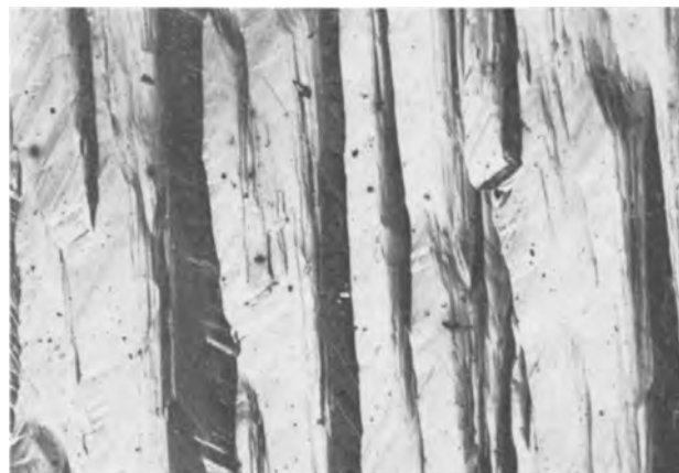
Fig. 1. Oriented growth on a (111) germanium surface after 16 hr at 885^{\circ}\text{C} . Magnification approximately 40x.
