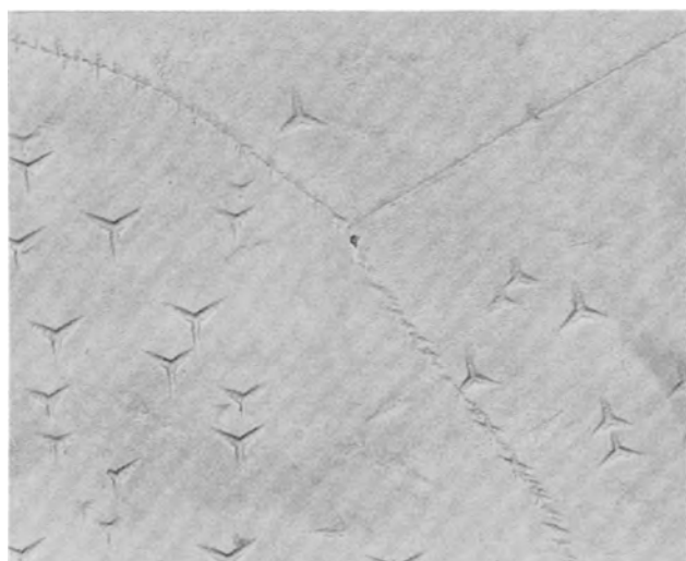
Fig. 10. Surface of tantalum heated 1 hr in argon at 800°C. 35,000X.
