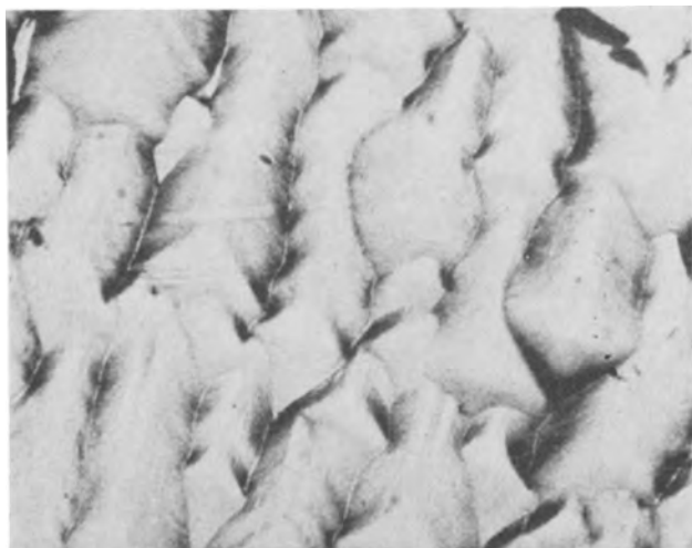
Fig. 5. Photomicrograph of a smooth part of a 50\mu thick electrodeposit. Magnification approximately 360X.
