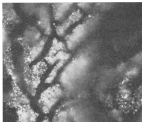
Fig. 4. Dark edge of a Mg electrode etched anodically in \text{HClO}_4 (Fig. 3). Shiny particles are present. Magnification 1430X.
