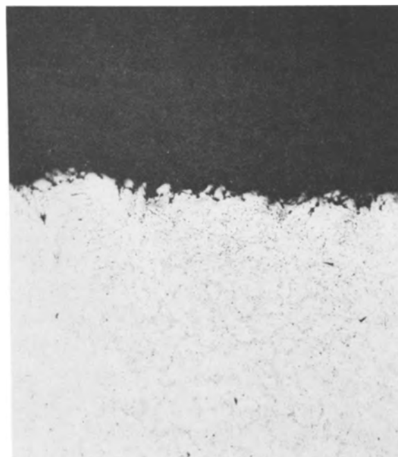
Fig. 4. Intergranular hot leg corrosion of Ti inhibited loop. Magnification 170X.
