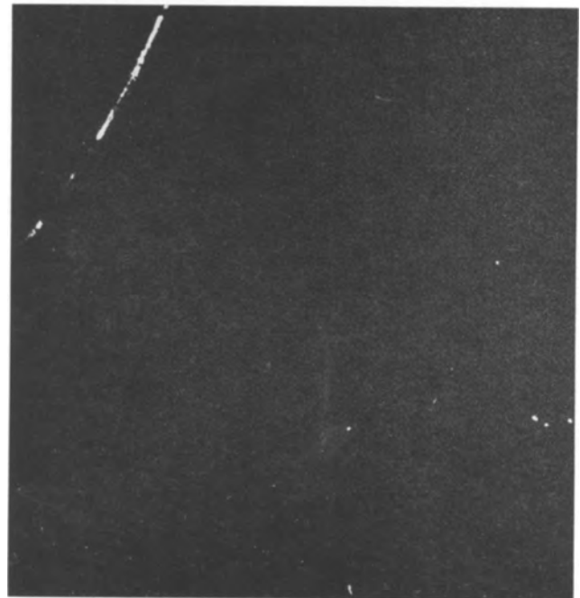
Fig. 15. Holes produced by 10-sec HF etch. Transmission through stripped film. 35,000X.
