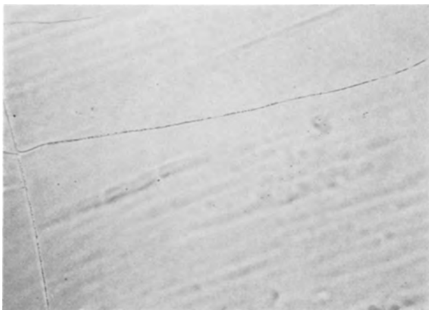
Fig. 24. Flaws (dark colored) in a reformed crack in a 3100Å film. 500X.
