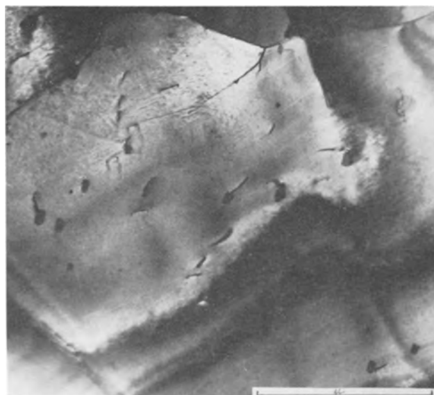
Fig. 8. Transmission electron micrograph of a tin-indium alloy foil after oxidation at 190°C and 10 torr for 2800 min.
