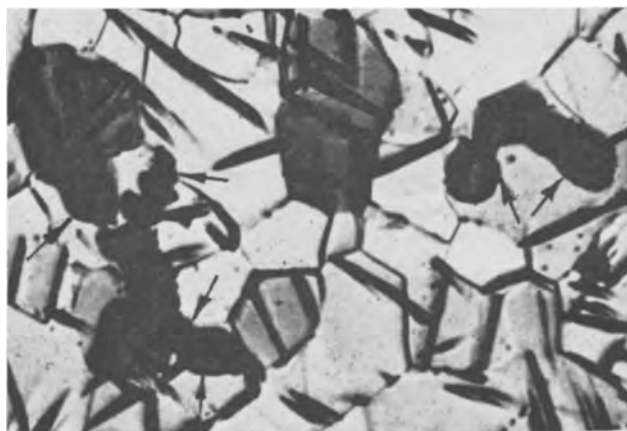
Fig. 24. Surface of Van Arkel zirconium, after 10 min in dry oxygen at 1 atm, 500°C showing "fronts" of thicker oxide. Magnification approximately 100X.
