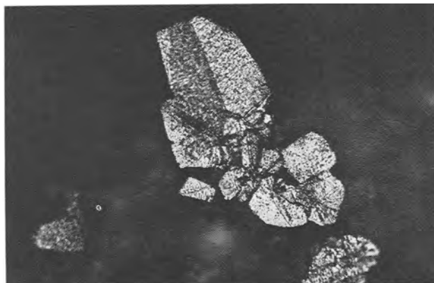
Fig. 3. Cross section of copper sponge showing twin planes
