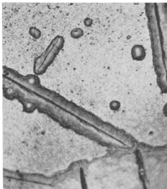
Fig. 21. Surface of Van Arkel zirconium after 17 hr at 1 atm and 1 hr at 500 psi in steam at 500°C. Magnification approximately 500X.
