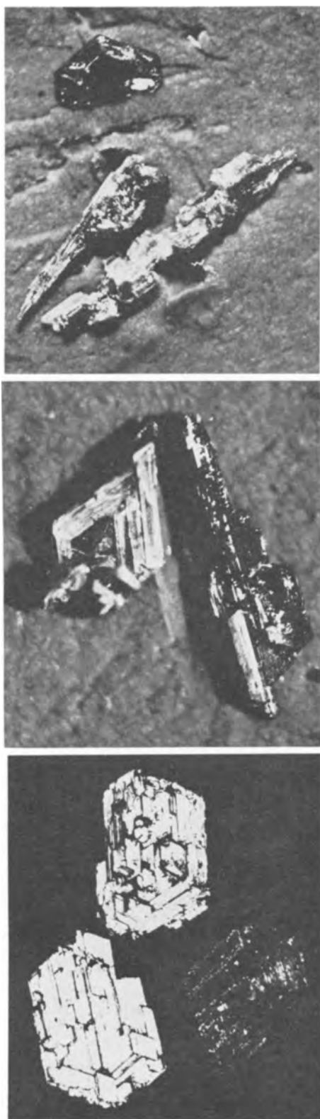
Fig. 1. Crystals of silicon carbide; Fig. 1a, top; Fig. 1b, center; Fig. 1c, bottom. Magnification 10X.
