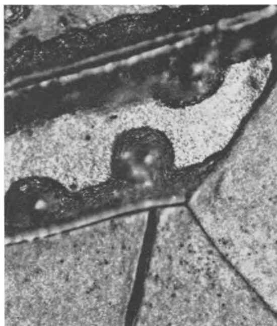
Fig. 22. Surface of Van Arkel zirconium after 14 hr at 1 atm and 4 hr at 500 psi in steam at 500°C. Magnification approximately 500X.
