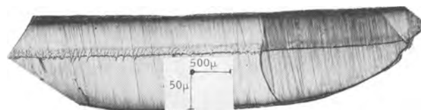
Fig. 14. Bevel-polished, gold plated lightly, and etched in 10:1:1::\text{H}_2\text{O}:\text{H}_2\text{O}_2:\text{HF} for 15 sec. Bevel slope is 0.1; X_j \sim 50\mu ; X'_j = 40\mu . \text{ZnAs}_2 diffused at 850^\circ\text{C} for 16 hr. Note that X'_j is constant in both grains, while X_j varies slightly, and that flatness is poorer in the main part of the crystal.
