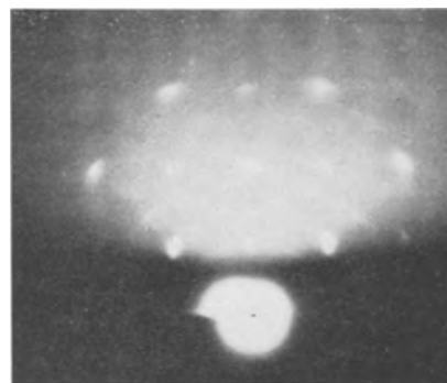
Fig. 7. Electron diffraction pattern of \text{CaTiO}_3 film, 570 Å thick, deposited at 550°C on LiF; azimuth [100]. (LiF spots visible).
