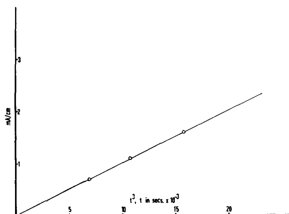
Fig. 1. Variation of current with cube of time for the electrodeposition of \gamma -manganese dioxide onto a platinum electrode at a potential E_h = 1320 mv. Solution composition: 0.01M MnSO_4 , 1.0M Na_2SO_4 , 0.25M H_2SO_4 .
